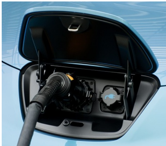
Nissan Leaf uses two connectors (DC-JARI and AC-J1772)
