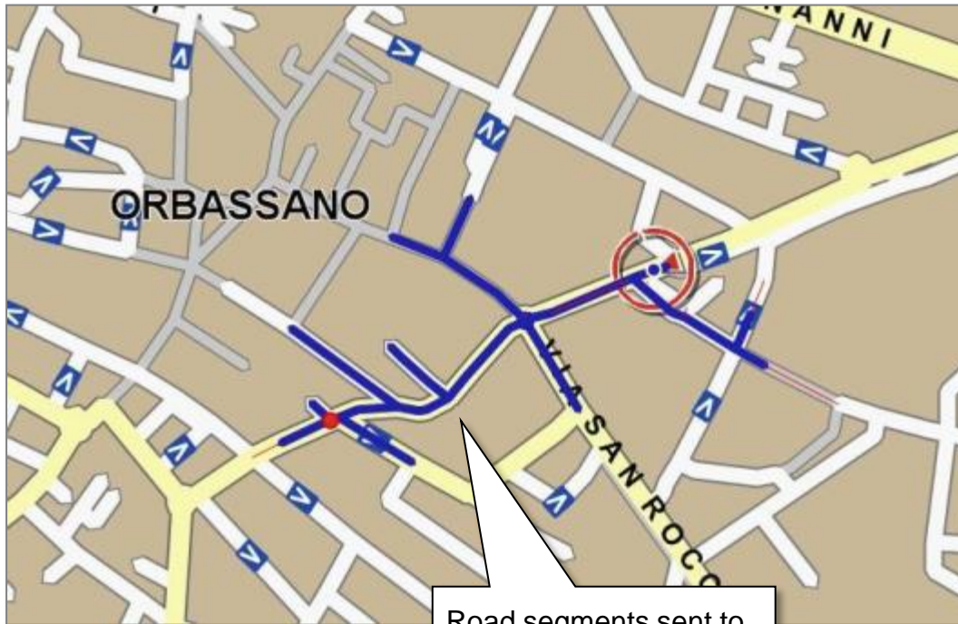
Typical path prediction by eHorizon provider
