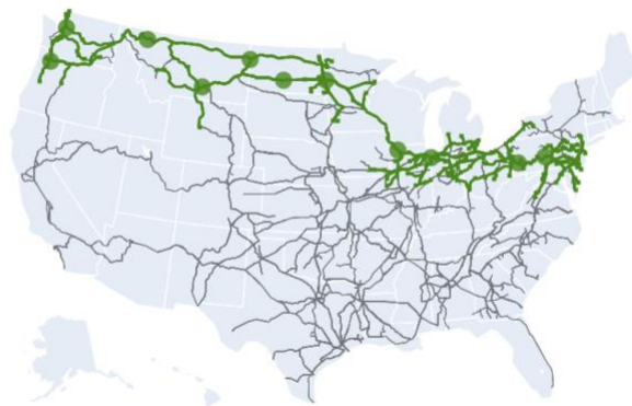
Figure 13 - Solution from Min Cost problem for battery-electric locomotives in 2025.
