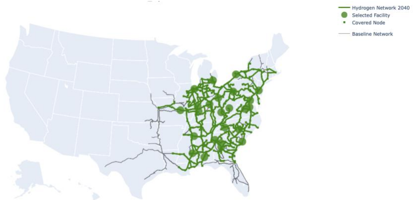
Figure 22 - Solution from Max Flow problem for hydrogen locomotives in 2040.
