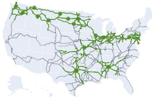
Figure 9 - Solution from Max Flow problem for battery-electric locomotives in 2035.
