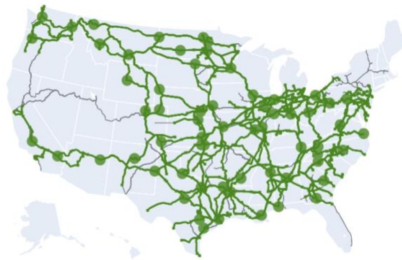
Figure 16 - Solution from Min Cost problem for battery-electric locomotives in 2040.
