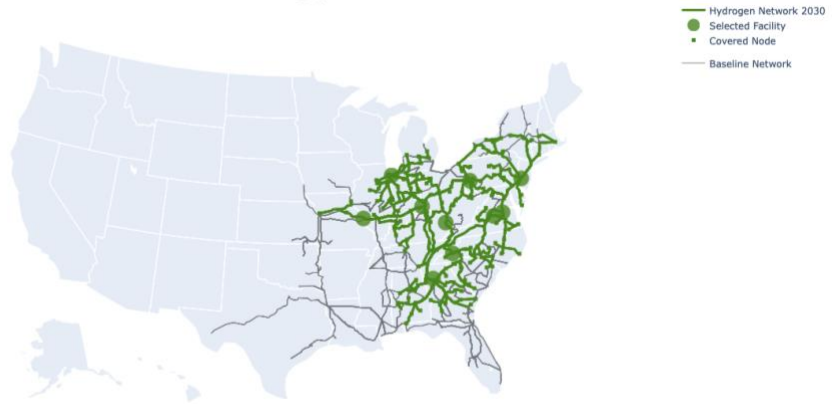
Figure 20 - Solution from Max Flow problem for hydrogen locomotives in 2030.
