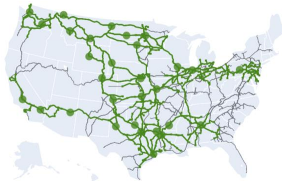
Figure 12 - Solution from Max Flow problem for battery-electric locomotives in 2050.
