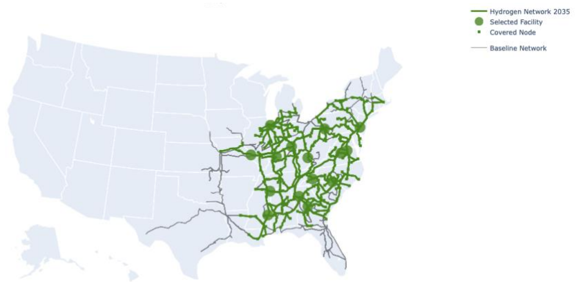
Figure 21 - Solution from Max Flow problem for hydrogen locomotives in 2035.
