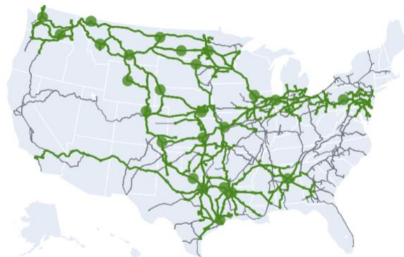
Figure 11 - Solution from Max Flow problem for battery-electric locomotives in 2045.
