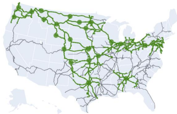
Figure 14 - Solution from Min Cost problem for battery-electric locomotives in 2030.
