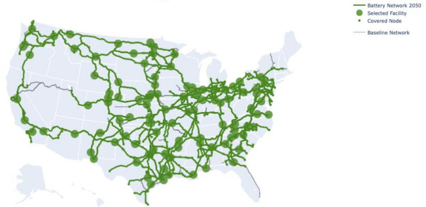
Figure 18 - Solution from Min Cost problem for battery-electric locomotives in 2050.
