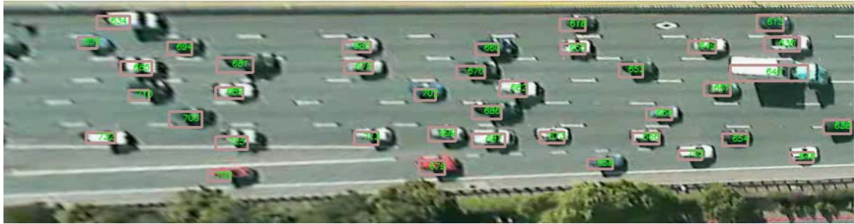
Figure 8 Example of traffic video being analyzed (red squares are tracking results of vehicles)
