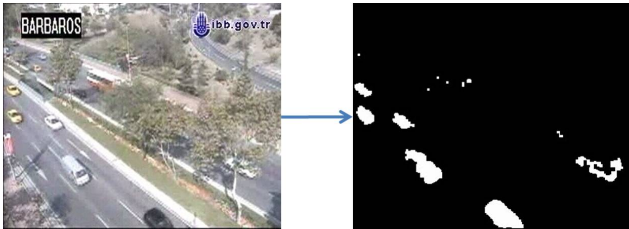
Figure 2 Left: An input video frame, Right: The result of the background subtraction module (foreground pixels are marked with white)
